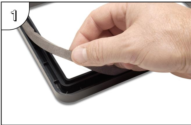
Start at one corner and pull the old gasket out of the channel that holds the gasket in place. Pull the gasket up as you work around the entire perimeter of the adapter plate. Discard the old gasket.
