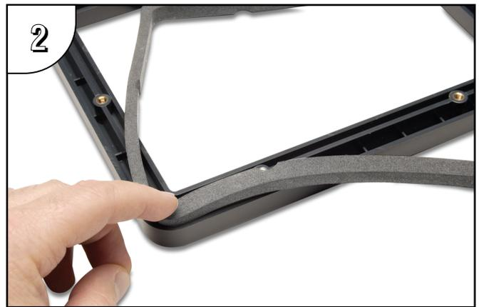
Lay the new gasket over the channel so that the long and short sides of the gasket match up to the long and short sides of the adapter plate. Start at one corner and match the gasket's corner to the channel's corner. Press the gasket into the channel and work all away around the perimeter of the adapter plate. Re-install the adapter plate and then the touch panel.
