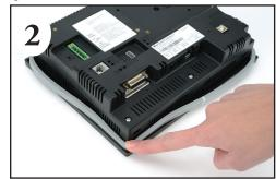
Lay the new gasket over the channel so that the long and short sides of the gasket match up to the long and short sides of the touch panel. Start at one corner and match the gasket's corner to the channel's corner. Press the gasket into the channel and work all away around the perimeter of the touch panel. Re-install the touch panel.
