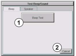
The internal Beeper can be tested from this system setup screen whether the Beeper is enabled or disabled. After the **Beep Test** button is pressed and released, the Beeper will sound for 500 msec.
