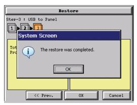
This message is displayed to indicate the **Restore** is complete. Press the **OK** button to return to the previous menu selection.
