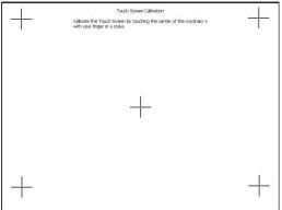
After pressing **OK**, the touch panel will reboot and startup on the **Touch Screen Calibration** procedure as shown here.
