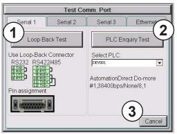
The following test can be used to check the operation of the serial communication ports, with the use of a loop back connector and can also check the serial communications to any connected and configured PLC.
