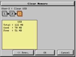
The data file(s)selected to clear are verified. If the data file is good, then the OK button can be pressed to start the clear procedure.
