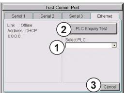
This function allows the ability to select any PLC configured in the project that may be connected to the touch panel through an Ethernet port connection and checks to see if the communications are working correctly.
