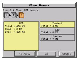
The data file(s)selected to clear are checked. If the data file is good, then the **OK** button can be pressed to start the clear procedure.
