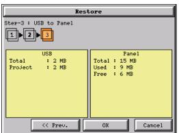
The data selected to restore is checked. If the data is good, then the **OK** button can be pressed to start the restore.
