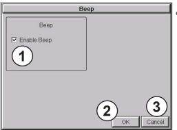
This system setup screen function is used to enable or disable the touch panel's internal beep function.
