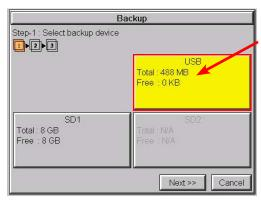
This is an example of selecting a USB memory device to write the backed up files to.
