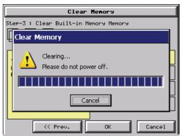
This message is displayed during the clearing process. Press the **Cancel** button to abort the clearing.
