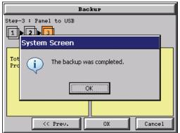
This message is displayed to indicate the **Backup** is complete. Press the **OK** button to return to the previous menu selection.
