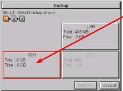
If the panel is powered up or rebooted with an SD card inserted into SD1 Slot, then the SD1 button's Total and Free memory will be displayed.
