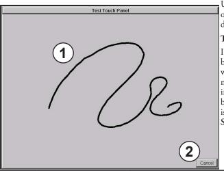
Using this test, normal or unusual operation of the analog touch panel can be determined.
