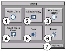
The **Setting Menu** is used to adjust the time & date, adjust the contrast or brightness of the display, enter the IP address settings, adjust (calibrate) the touch screen, enable or disable the internal beep and turn on and off the mouse cursor .
