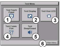
The **Test Menu** gives the user the ability to test the operation of the touch screen, test the LCD display, test the various communication ports, and also test the internal beeper and the audio line out through an user supplied amplified (stereo) speaker(s).
