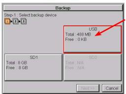
The Memory - Backup selection allows you to backup the panel's **Project**, **Log** files, **Recipe** files or even the **Firmware** files to either an SD memory card or **USB** pen drive. The available memory devices will be displayed with their total and free memory.
