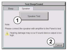
The **Speaker Test** function requires that a speaker(s) with an amplifier (can be stereo) be connected to the Audio Line Out stereo jack on the rear of the touch panel.
