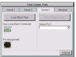
This function allows the ability to select any PLC that may be connected to the touch panel through the selected serial comm. port connection and checks to see if the communications are working correctly.
