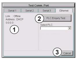
The following test feature can be used to check the operation of the Ethernet communication port by indicating if an Ethernet link has been established or not, and can also check the status of the Ethernet communications to any connected PLC.
