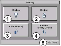
The user's project, Firmware and OS, log and recipes files can be backed up to or restored from an SD memory card (SD Card Slot 1 or SD Card Slot 2), or a USB memory device. From this menu the user can also clear the project log files. The user also has the ability to clear the memory within the *C-more* touch panel.
