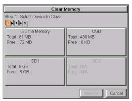
This function is used to clear individually selected data files, or all data files, within the panel's **Built-in Memory**, or any installed memory device such as a USB pen drive or an SD card.
