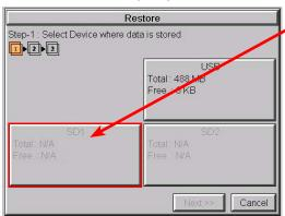
SD1 may be unavailable (grayed out) if there is no card in SD Slot 1 or the card in SD slot 1 has the project currently running on the panel stored on it.
