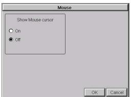
This system setup screen function is used to enable/ disable the arrow mouse cursor on the panel screen. It may be valuable to display the mouse cursor, for example, when an external USB keyboard is connected to the panel..
