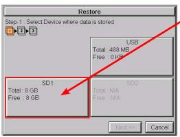
If the panel is powered up or rebooted with an SD card inserted into SD1 Slot, then the SD1 button's Total and Free memory will be displayed.
