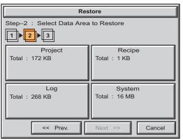
Select the data file(s) to be restored by pressing the appropriate data file button. The selection will be highlighted. The data file can be either the **Project**, **Firmware** and/or **Recipe files**. The selected data is restored to the internal built-in memory if there is no SD card inserted into the SD1 slot.
