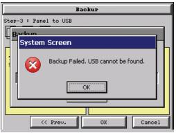
This warning message will be displayed if the backup Memory device fails or is removed during the backup. Press the OK button to clear the warning message.
