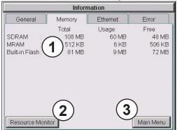
1. **Memory components** - Status of each memory component - SDRAM, MRAM and Built-in Flash are internal memory components. When external memory devices are installed in the panel they will be included in this list: SD1, SD2 (12 and 15 inch panels only) and USB.
