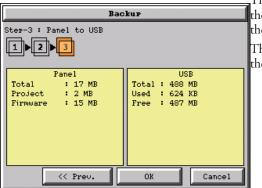
The next system setup screen allows the verification of the data file selections. When the OK button is pressed, the backup begins.
