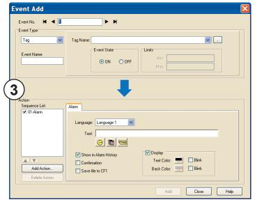
Click on the Tag Name: pull down menu and select the internal System Bit On (SYS BIT ON) tag as shown. This will force the tag event type to be continuously active.
