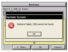
This warning message will be displayed if the restore Memory device fails or is removed during the backup. Press the **OK** button to clear the warning message.
