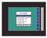
**Serial Port - Loop Back Test** - Performs a test to verify either the RS-232 or the RS485/422 serial communications functionality from the 15-pin connector (Port 2) on the panel is operating correctly. A loop back connector inserted into the port is required for proper testing. Wiring diagrams to build RS-232 and RS-485/422 loop back connectors are shown below.
