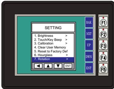
With Rotation highlighted, press ENT [F5] to show the current orientation. Press UP [F3] and DWN [F4] to toggle between the portrait (vertical) and landscape (horizontal) orientation. Use the APL [F5] function button to apply the selection.
