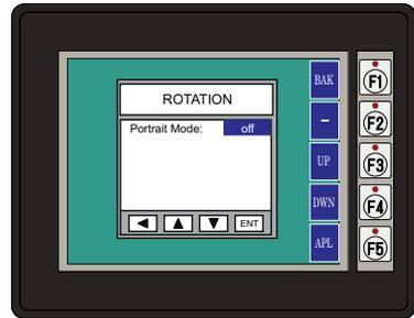
**Note:** Loading a project to the panel will override the orientation chosen from the System Setup Screens' Rotation selection screen. The selected orientation is displayed only when in the System Setup Screens.
