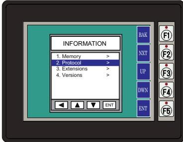
Pressing ENT [F5] with **Protocol** highlighted will show the PLC Protocol that has been assigned to the panel and the protocol version.
