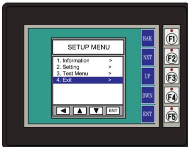
Pressing ENT [F5] with **Exit** highlighted will allow the user to decide whether to **Exit** or not **Exit** the System Setup Screens. See page 5-18.
