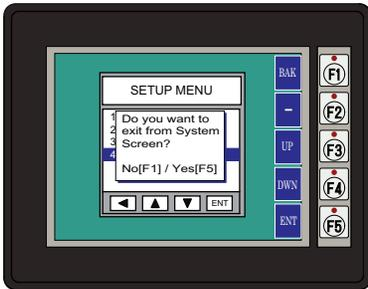
With **Exit** highlighted, press ENT [F5] to bring up the screen shown to the left. You will be given the choice to either proceed with exiting the **System Setup Screens** by pressing [F5] for YES or allowed to cancel by pressing [F1] for NO. You will be returned to the project screen if answering YES.
