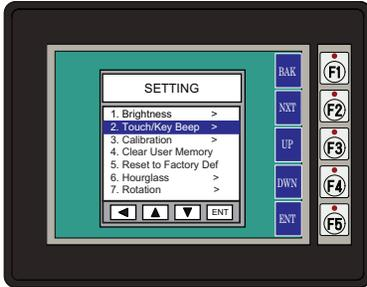
With Touch/Key Beep highlighted, press ENT [F5] to show the current value for the internal beeper. The default is ON. The UP [F3] and DWN [F4] function keys can be used to toggle between the ON and OFF state for the beeper (enable or disable). Use the APL [F5] function key to apply the selection.
