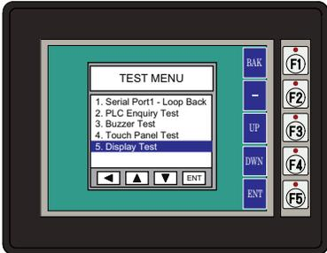
With Display Test highlighted, press ENT [F5] to bring up the screen shown to the right. After a few seconds a scrolling RGB color test will begin. Use this test to identify any area that is displaying colors incorrectly. Press any key [F1 to F5] to return to the Test Menu.
