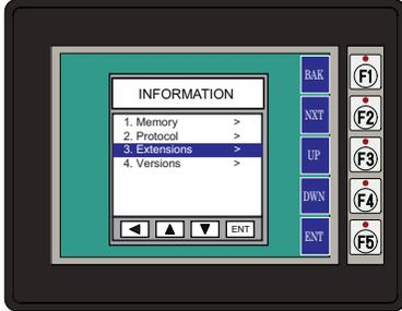
Pressing ENT [F5] with **Extensions** highlighted will show if an optional keypad bezel is installed on the panel. The example here shows the EA-MG6-BZ2.
