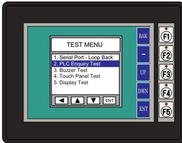
With **PLC Enquiry Test** highlighted, press ENT [F5] to bring up the screen shown to the right. If the PLC is connected to the panel, press ENT [F5] to start the test. Four data tests will be performed and indicated as either **Test Passed** or **Test Failed** as shown on this page. The BAK [F1] key can be pressed to cancel the test and/or returned to the previous screen.
