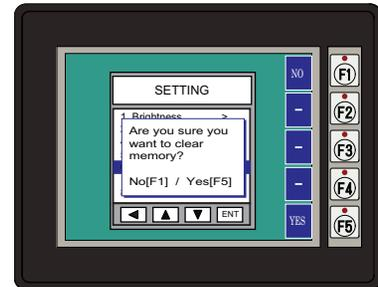
Factory default values can also be reset by pressing F2 and F4 while cycling power to the panel. The Factory Default values are:
