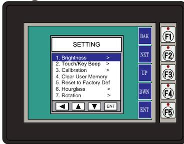
Use the UP [F3] and DWN [F4] function keys to scroll through the list of settings. The BAK [F1] function key will return you to the previous screen. Use the ENT [F5] function key to make your selection once you have the setting highlighted.
