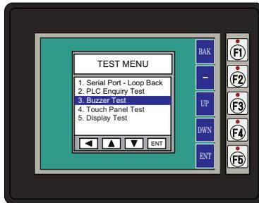
With **Buzzer Test** selection highlighted, press ENT [F5] to run the test on the internal audible beeper. The beeper will sequence up the scale through eight notes and then start over. The BAK [F1] key can be pressed to cancel the test.
