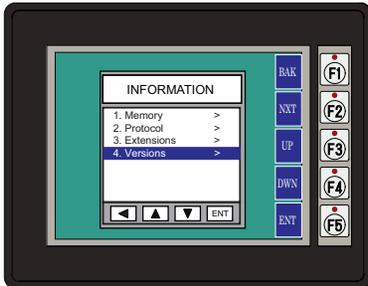
Pressing ENT [F5] with **Versions** highlighted will show the panel model, firmware and boot loader versions.\*
