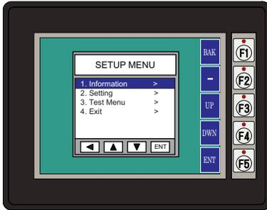
To navigate the different selections under the Setup Menu, use the function keys BAK [F1] to return to the project screen or previous screen, UP [F3] to cursor up, DWN [F4] to cursor down, and ENT [F5] to enter a selection.
