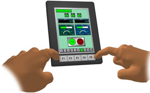
From the Setup Menu, information about the panel can be obtained, settings can be adjusted, and panel functions can be tested.
