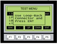
constructed as shown here and press ENT [F5] to start the test. If the test is passing, the Receive Counts will equal the Bytes Sent. If the serial then the Error Counts will equal test will continue until the BAK [F1] key is pressed.
