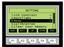
With Beep highlighted, press ENT [F5] to show the current value for the internal beeper. The default is ON. The UP [F3] and DWN [F4] function keys can be used to toggle between the ON and OFF state for the beeper (enable or disable). Use the APL [F5] function key to apply the selection.
