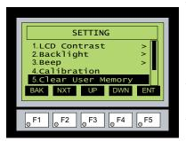
With Clear User Memory highlighted, press ENT [F5]. You will be given the choice to either proceed with clearing the user memory by pressing [F5] for YES or allowed to cancel by pressing [F1] for NO.
