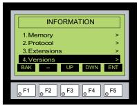
Pressing ENT [F5] with the **Versions** highlighted will show the panel model, firmware and boot loader versions.
