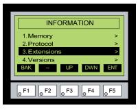
Pressing ENT [F5] with the Extensions highlighted will list the optional keypad bezel and/or DC power adapter that are installed on the panel. The example here shows the EA-MG-P1 & EA-MG-BZ1.
