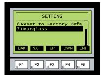
The Hourglass selection listed under the Setting menu can be used to either disable the display of the hourglass icon or set the amount of delay time (0 ms to 1000 ms) desired before it is displayed.
