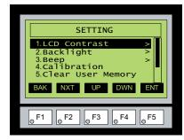
With LCD Contrast highlighted, press ENT [F5] to bring up the screen showing the current value. The default is a value of 3. The contrast can be adjusted between 1 to 5, with 1 being the least amount of contrast and 5 being the highest amount.
