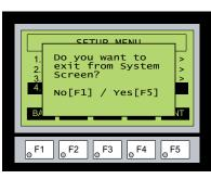
With Exit highlighted, press ENT [F5] to bring up the screen shown to the left. You will be given the choice to either proceed with exiting the System Setup Screens by pressing [F5] for YES or allowed to cancel by pressing [F1] for NO. You will be returned to the project screen if answering YES.
