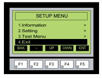
Pressing ENT [F5] with Exit highlighted will allow the used to decided whether to Exit or not Exit the System Setup Screens. See page 5-15.
