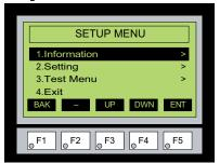
To navigate the different selections under the Setup Menu, use the function keys. BAK [F1] to return to the project screen or previous screen, UP [F3] to cursor up, DWN [F4] to cursor down, and ENT [F5] to enter a selection.
