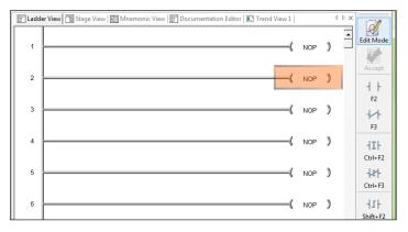
If multiple views are open in the Program display window at the same time, the tabs will appear as in the illustration below.
