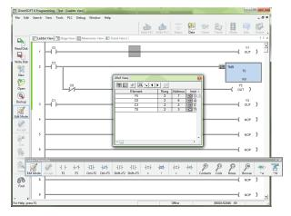
All docked views/toolbars can also be Floating views/toolbars, and float outside the application frame (very handy if multiple monitors are being used). The remaining area, bounded by all of these docked views/toobars, is where the primary MDI Views are positioned.
