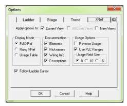
The other two sections located in the dialog, **Display Mode** and **Usage Options**, contain options that can be selected on the XRef View toolbar. Also notice the box to the left of the **Follow Ladder Cursor** option under the Display column. The box can be checked in this dialog or selected at will in the XRef Toolbar which is explained on the facing page.
