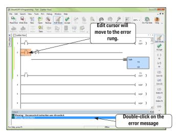
The Output window will appear below the view being displayed, in this case, the Ladder View. Each mistake or error message will be listed. Double-clicking on the error in the Output window will move the edit cursor to the error rung in the ladder view. Once all of the errors are corrected, the program can be compiled. The error messages in the Output window will disappear but the window will remain in view as can be seen in the diagram on the facing page.
