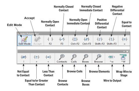
The contact buttons are self-explained. Each contact button will place the particular element on the rung wherever the edit cursor is placed.
