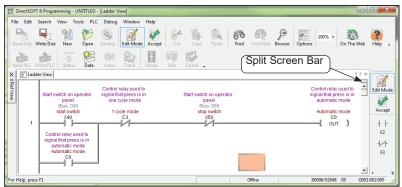
This diagram illustrates the split screen. Notice that the lower pane is showing a different rung than the upper pane.
