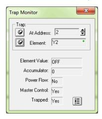
If you want to "step" through a program area to check the data in V-memory locations, just leave the Trap Monitor dialog as shown above, then place the ladder program cursor over the element (box) with the memory reference in it. You can then read the data in the read only area.
