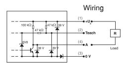
U<sub>B</sub> 10 ... 30 VDC I<sub>Δ</sub> 200 mA max.
