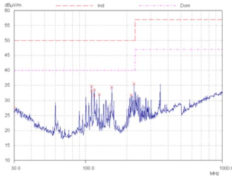
emissions in region of 30-1000MHz are observed. The products are set up in a real life situation, with appropriate cables, industrial enclosure etc. To the left is an example of a radiated emissions scan. The two limit lines shown are domestic and industrial, and are only relevant to a test distance of 3 metres. Although the accuracy of a good anechoic chamber is high, the standards still stipulate the use of an
