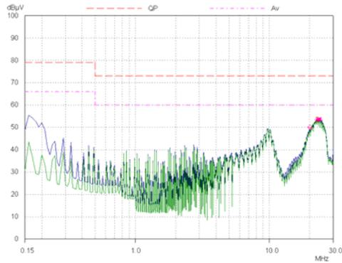
The test is carried out within the anechoic chamber, and a LISN (line impedance stabilisation network) is used to couple the product to the mains supply. The LISN has an rf pickup socket which is used to output the rf signal to the test receiver, where a scan is run. Two scans are run, one between line and earth and the other between neutral
