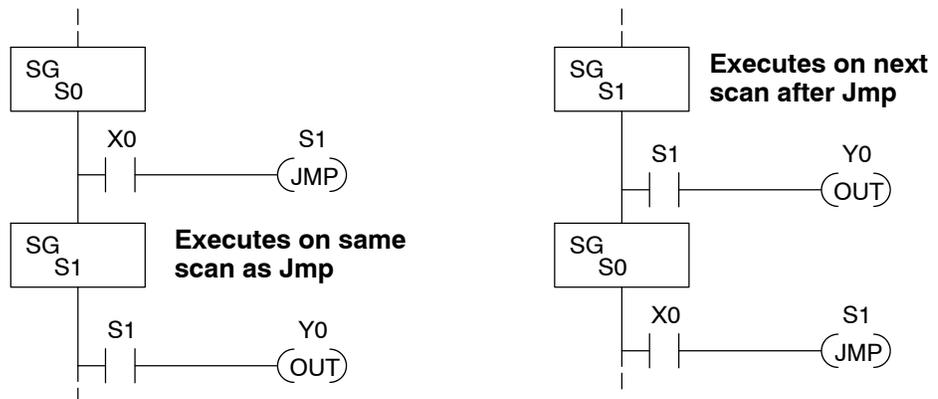
**NOTE:** Assume we start with Stage 0 active and Stage 1 inactive for both examples.
