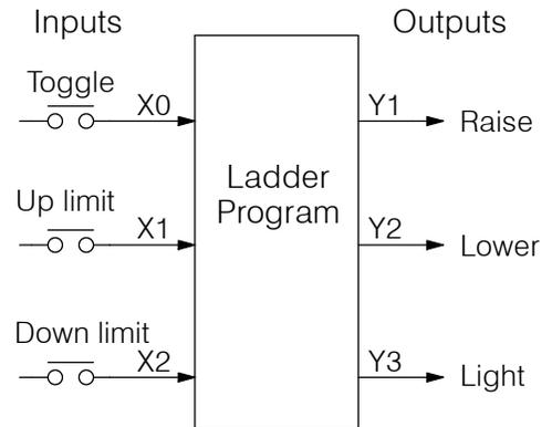
We can think of the Light state as a parallel process to the raise and lower state. The paths to the Light state are not a transition (Stage JMP), but a State Set command. In the logic of the Light stage, we will place a three-minute timer. When it expires, timer bit T0 turns on and resets the Light stage. The path out of the Light stage goes nowhere, indicating the Light stage just becomes inactive, and the light goes out!
