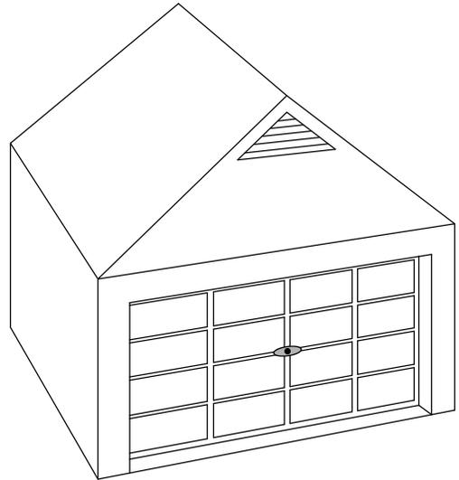
In order to identify the inputs and outputs of the system, it's sometimes helpful to sketch its main components, as shown in the door side view to the right. The door has an up limit and a down limit switch. Each limit switch closes only when the door has reached the end of travel in the corresponding direction. In the middle of travel, neither limit switch is closed.
