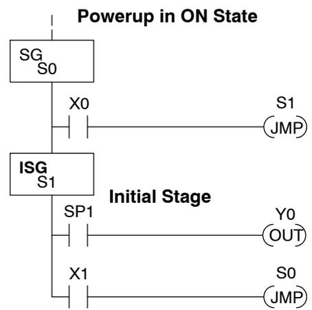
**NOTE:** If the ISG is within the retentive range for stages, the ISG will remain in the state it was in before power down and will NOT turn itself on during the first scan.
