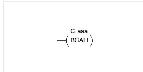
**Must Remain Active** — The BCALL instruction actually controls all the stages between the BLK and the BEND instructions even after the stages inside the block have started executing. The BCALL must *remain* active or all the stages in the block will automatically be turned off. *If either the BCALL instruction, or the stage that contains the BCALL instruction goes off, then the stages in the defined block will be turned off automatically.*
