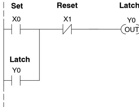
When the Off pushbutton (X1) is pressed, it opens the normally-closed X1 contact, which **resets the latch**, and output Y0 turns off.
