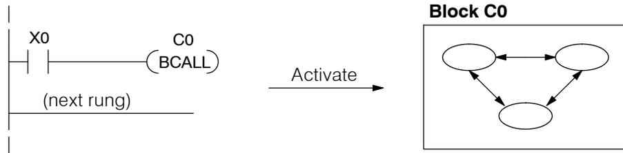
When a stage block becomes active, the first stage in the block automatically becomes active on the same scan. The “first” stage in a block is the one located immediately under the block (BLK) instruction in the ladder program. So, that stage plays a similar role to the initial type stage we discussed earlier.
