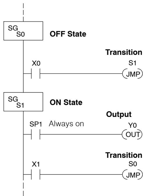
For now, let's assume we begin in the OFF State, so stage S0 is active. When the On pushbutton (X0) is pressed, a stage transition occurs. The JMP S1 instruction executes, which simply turns off the Stage bit S0 and turns on Stage bit S1. So on the next PLC scan, the CPU will not execute Stage S0, but will execute stage S1!
