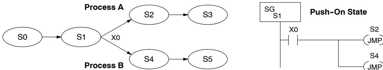
Note that if we want Stages S2 and S4 to energize exactly on the same scan, both stages must be located below or above Stage S1 in the ladder program (see the explanation at the bottom of page 10-7). Overall, parallel branching is easy!
