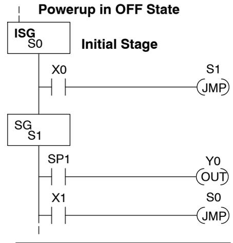
We can change both programs so that the motor is ON at powerup. In the RLL below, we must add a first scan relay SP0, latching C0 on. In the stage example to the right, we simply make Stage S1 an initial stage (ISG) instead of S0.
