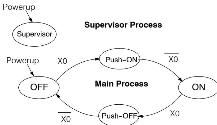
New stage programming students will typically try to place the counter inside one of the the stages of the process they are trying to monitor. The problem with this approach is that the stage is active only part of the time. In order for the counter to count, the count input must transition from off to on at least one scan after its stage activates. Ensuring this requires extra logic that can be tricky.
