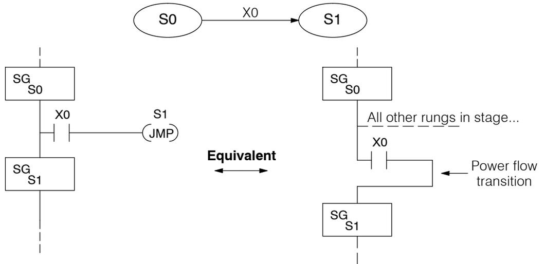
Recall that the Stage JMP instruction may occur anywhere in the current stage, and the result is the same. However, power flow transitions (shown above) must occur as the last rung in a stage. All other rungs in the stage will precede it. The power flow transition method is also achievable on the handheld programmer, by simply following the transition condition with the Stage instruction for the next stage.
