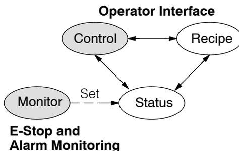
**How Instructions Work Inside Stages** We can think of states or stages as simply dividing up our ladder program as depicted in the figure below. Each stage contains only the ladder rungs which are needed for the corresponding state of the process. The logic for transitioning out of a stage is contained within that stage. It's easy to choose which ladder rungs are active at powerup by using an "initial" stage type (ISG).
