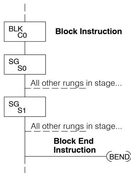
Note that the stages within a block must be regular stages (SG) or convergence stages (CV). So, they cannot be initial stages. The numbering of stages inside stage blocks can be in any order, and is completely independent from the numbering of the blocks.
