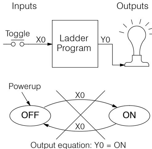
Note that this example differs from the motor example, because now we have just one pushbutton. When we press the pushbutton, both transition conditions are met. We would just transition around the state diagram at top speed. If implemented in Stage, this solution would flash the light on or off each scan (obviously undesirable)!
