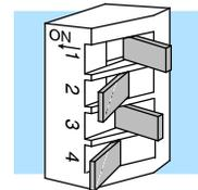
**Remember:** You must set Pos.4 of the DIP switch to ON in order for discrete addressing to be available.
