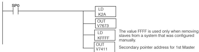
**NOTE:** Remember, when you determine the bit pattern value for **automatic slave removal**, you have the option of merely setting Bit 0. This would indicate that you want *any* slave to drop out when it causes a communications error. If you do this, then you won't have to set each slave bit individually. In the above example, we only remove slaves 1, 3, and 5. Therefore, we decided not to use Bit 0. We instead set Bits 1, 3, and 5 which resulted in the value HEX 2A.
