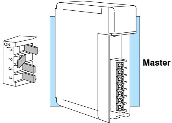
The settings of pos.1 and pos.2 of the slaves must match the ON/OFF state of these same positions on the master module's DIP switch. Otherwise, they will be set at different baud rates and will not be able to communicate.
