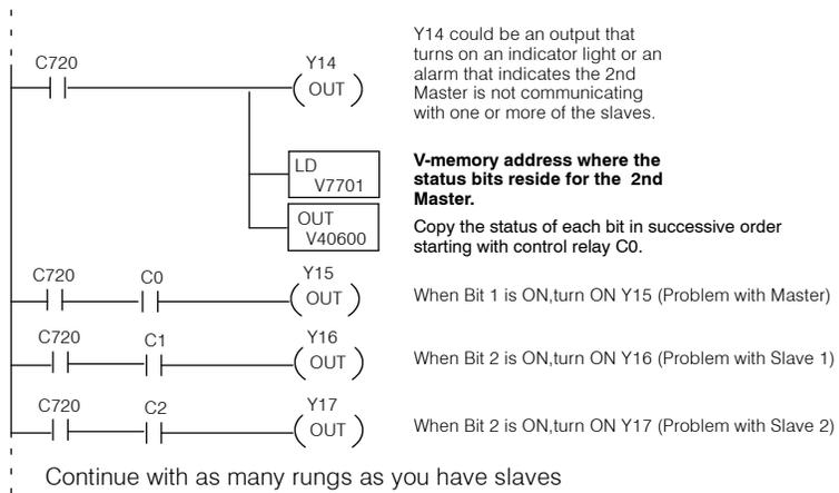
Bit 0 is used to indicate a problem with the master, so the first control relay that contains slave information is C1. Also, notice how the control relays do not match up with the slave number after bit 7. This is because the control relays are numbered in octal, not decimal. For example, you'll notice that slave 9 is represented by C11.
