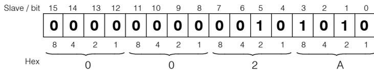
Since the Bit number is the same as the Slave number, it is easy to know which bits to set. Once you set these bits, you can convert the binary value to hex. Notice how bits 1 and 3 result in 10, which is hex A.
