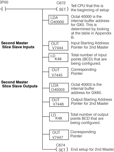
**Note:** From a point of consistency, you might prefer to manually configure the Slice I/O for both Masters. This example is for illustration only.
