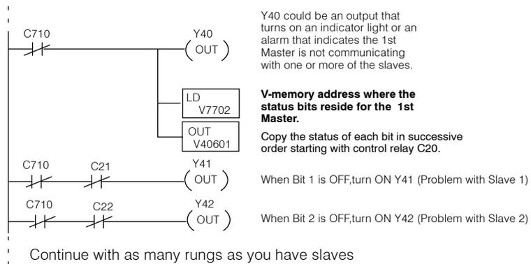
**Note:** C20 is not used here because the first bit does not mean anything for the mapping check.
