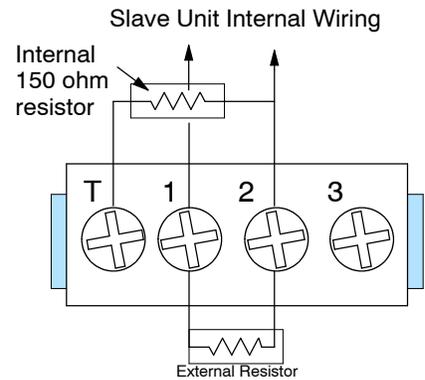
You add your own resistor, using a resistor between 100 and 300 ohms to match the impedance of the cable.
