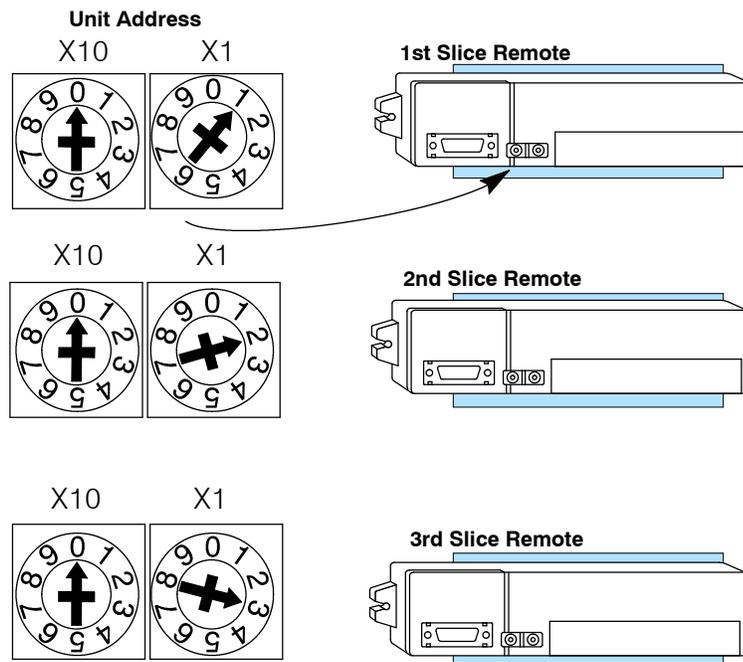
Align the arrow on the switch to any numbers between 01 and 15 (decimal), depending on which slave in sequence you are setting up and how many slaves are allowed per master. Remember, each addressing mode (automatic, manual and discrete) has a particular limit on how many slaves can be connected to the master.
