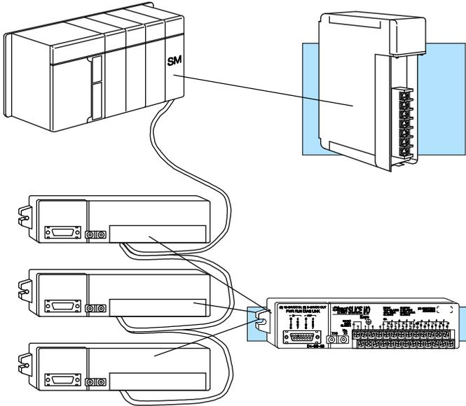
**Slice Master** -The D4-SM can link up to 15 Slice slaves (using discrete addressing) per master module. It is mounted in the CPU base. Up to 2 masters can be used.
