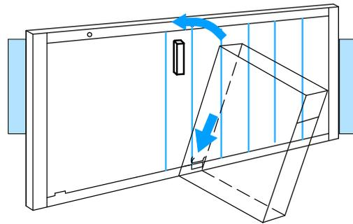
The master can go into any slot in the local base.
