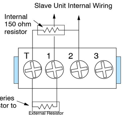
You add your own resistor in series with the 150 ohm internal resistor to match the cable impedance.
