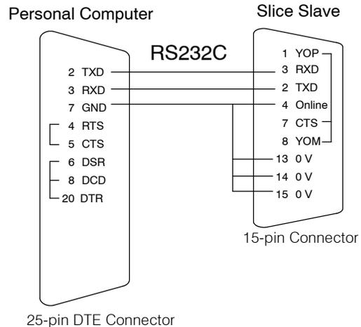
Pin labeling conforms to the IBM DTE and DCE standards.
