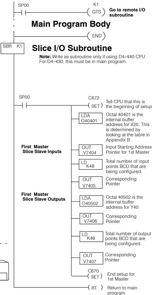
**Note:** V-memory pointer for 1st Master inputs start at V7404 with number of points being transferred in V7405. The output pointer starts at V7406 with number of points being transferred in V7407.
