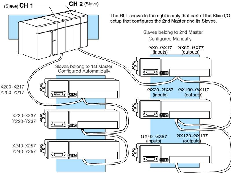
Setting C672 tells the CPU that this is the beginning of the Slice I/O configuration setup.
