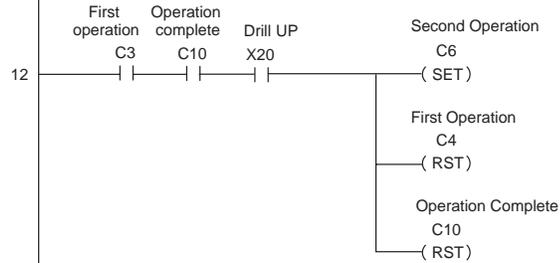
With the second drilling operation is complete, the drill is in the raised position, and the part is removed, reset C6 and C10 and enable the logic that invokes Home Search by pulsing C11.
