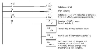
You should probably take note that Ym +21 does not have to stay ON. If Ym +21 is turned OFF, the sampling process would continue until completion anyway.
