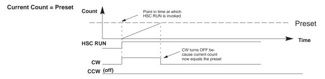
There may be occasions when you are counting down towards a preset. For example, you may have loaded a negative preset, or, you may have used an offset to change the current count so that it is above the preset. The following diagram shows how the HSC can also automatically control the counter clockwise (CCW) output.
