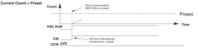
As the current count continues to approach the preset, the HSC will monitor the relationship between the current count and the preset. When the current count is equal to the preset, the HSC automatically turns off the clockwise output (CW).
