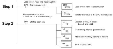
**NOTE:** Preset may be loaded at any time, but it is not accepted by the HSC until the HSC run bit transitions from off to on.
