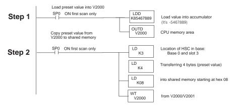
Notice that we loaded an 8-digit number with an 8 as the first digit. Remember you are loading a BCD number and not a decimal value. Remember that the MSB is always "8" when you are writing a negative number.
