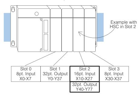
The HSC module will *automatically* consume 16 inputs and 32 outputs. The table on Page 5 of this chapter shows you how the HSC X's and Y's are assigned to specific functions.
