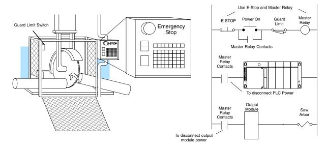
After an Emergency shutdown or any other type of power interruption, there may be requirements that must be met before the PLC control program can be restarted. For example, there may be specific register values that must be established (or maintained from the state prior to the shutdown) before operations can resume. In this case, you may want to use retentive memory locations, or include constants in the control program to ensure a known starting point.
