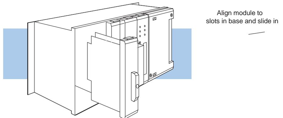
**WARNING:** Never connect or install a module into the base while the power is applied. Failure to remove the power prior to the installation can result in damage to the module, other installed modules, the power supply and/or the CPU itself.
