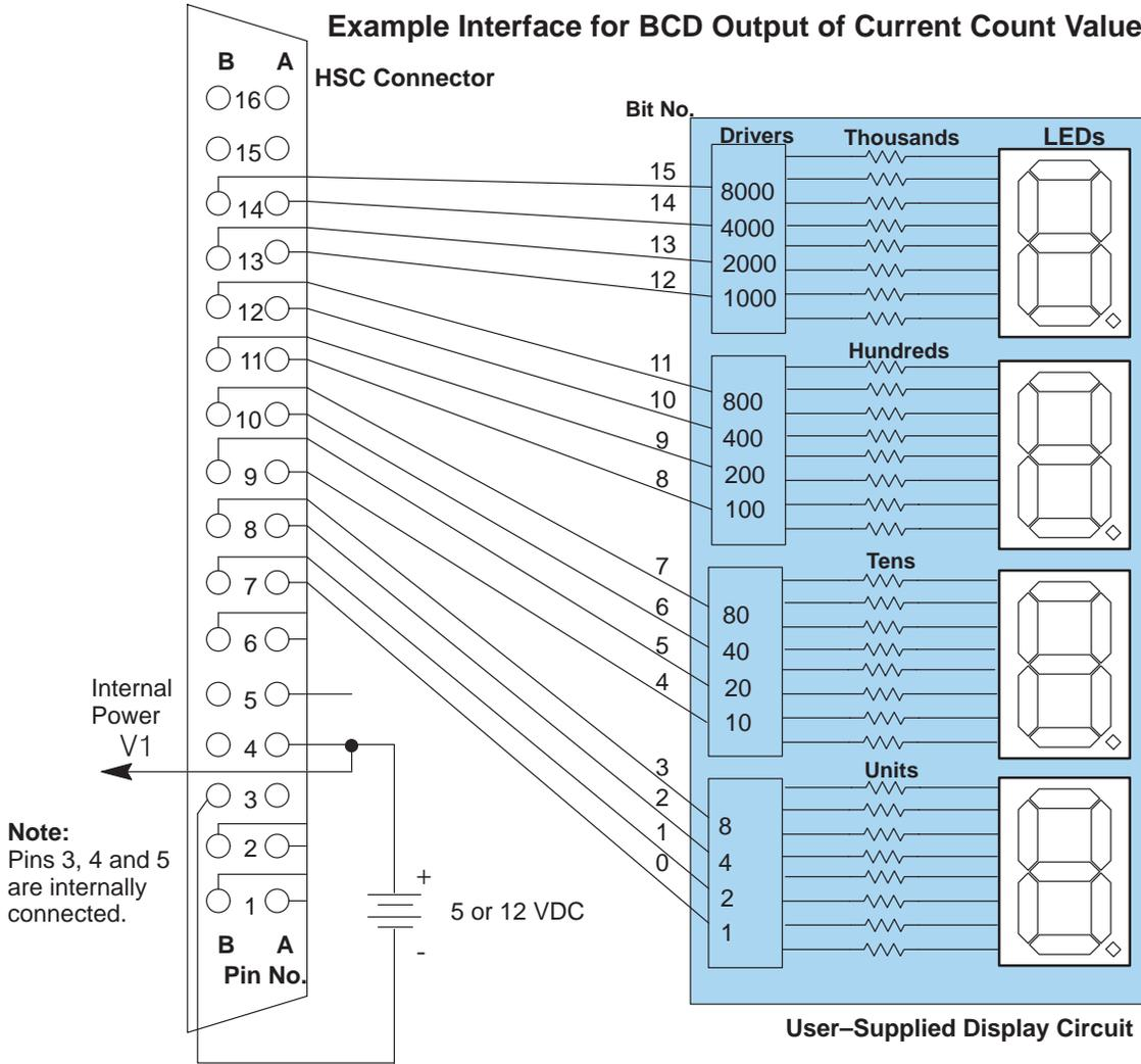
**BCD Output Circuit (For Interfacing Display Device or Input Module)**
