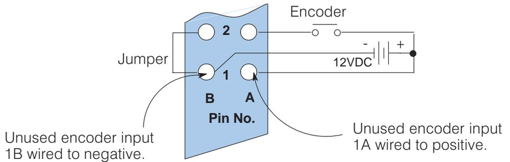
**NOTE:** There are two pairs of encoder connecting pins. 1A and 1B are for UP counting and 2A and 2B are for DOWN counting. You must hook your encoder to one set of pins. The unused set of pins must have the (A) pin connected to the positive side of the encoder supply, and the (B) pin connected to the negative side.
