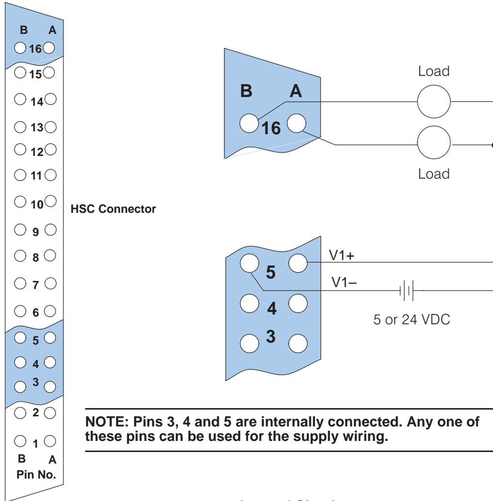
**NOTE:** Pins 3, 4 and 5 are internally connected. Any one of these pins can be used for the supply wiring.
