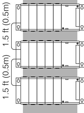
8 slot local CPU base with a 5 slot expansion base
