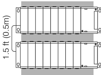
8 slot local CPU base with two 8 slot expansion bases
