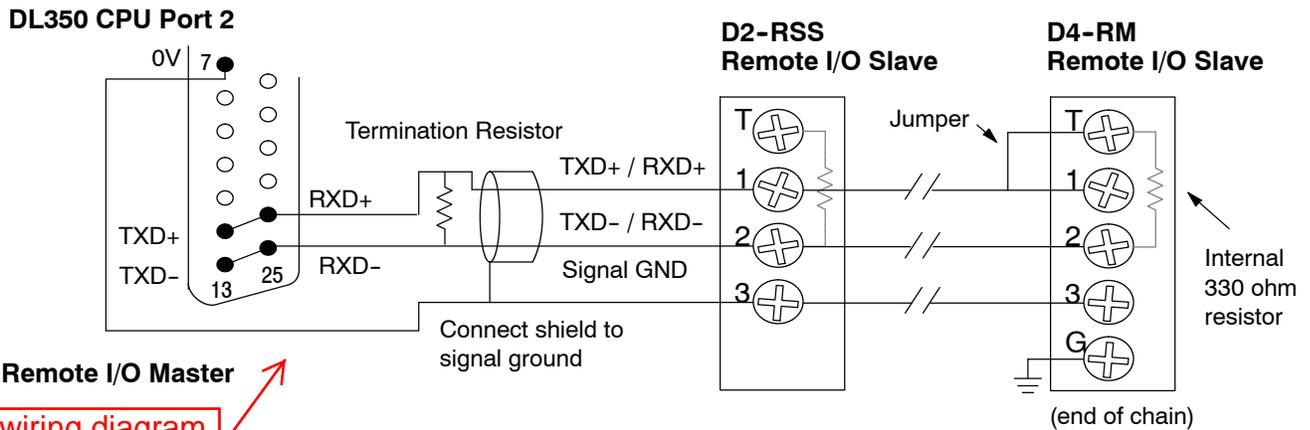
This wiring diagram is incorrect. Refer to the wiring diagram shown on the Errata Sheet on the first page of this file.
