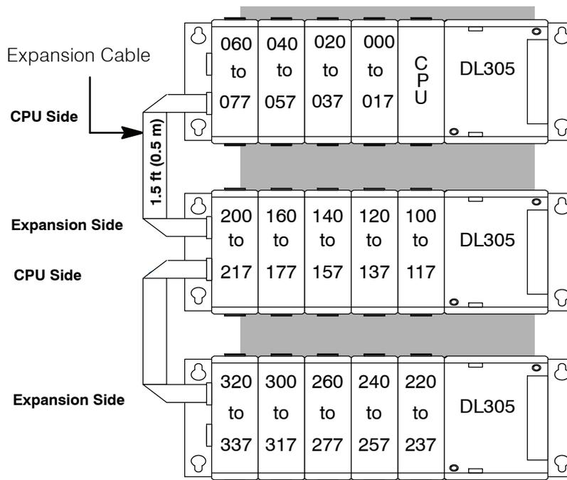
Note: Avoid placing the expansion cable in the same wiring tray as the I/O and power source wiring.
