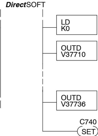
On the last rung in the example program above, we set a special relay contact C740. This particular contact indicates to the CPU the ladder program has finished specifying a remote I/O system. At that moment the CPU begins remote I/O communications. Be sure to include this contact after any Remote I/O setup program.
