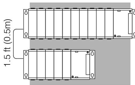
10 slot local CPU base with a 10 slot expansion base
