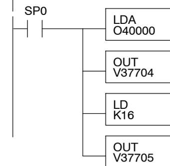
Consider the simple system featuring Remote I/O shown below. The DL350's built-in Remote I/O channel connects to one slave base, which we will assign a station address=1. The baud rates on the master and slave will be 38400 kB.
