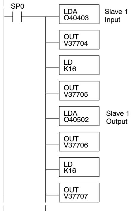
When configuring a Remote I/O channel for fewer than 7 slaves, we must fill the remainder of the table with zeros. This is necessary because the CPU will try to interpret any non-zero number as slave information.
