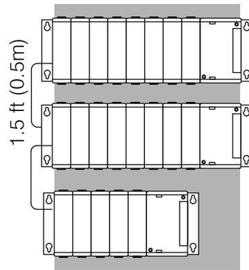
8 slot local CPU base with a 8 slot expansion base
