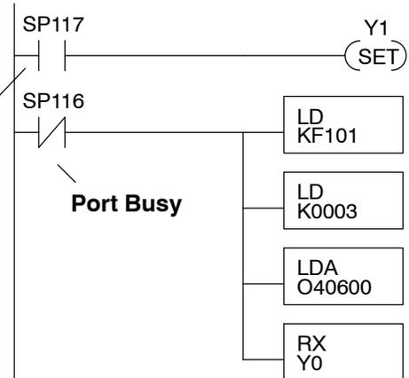
The port which can be a master has two Special Relay contacts associated with it (see Appendix D for comm port special relays). One indicates “Port busy”(SP116), and the other indicates “Port Communication Error” (SP117). The example above shows the use of these contacts for a network master that only reads a device (RX). The “Port Busy” bit is on while the PLC communicates with the slave. When the bit is off the program can initiate the next network request.
