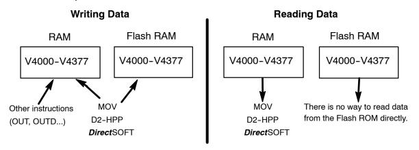
After a power cycle, the PLC always copies the data in the flash ROM to the RAM. If you use the instructions except for the MOV instruction to write data into the non-volatile V-memory area, you only update the data in RAM. After a power cycle, the PLC copies the previous data from the flash memory to the RAM, so you may think the data you changed has disappeared. To avoid trouble such as this, we recommend that you use the MOV instruction.
