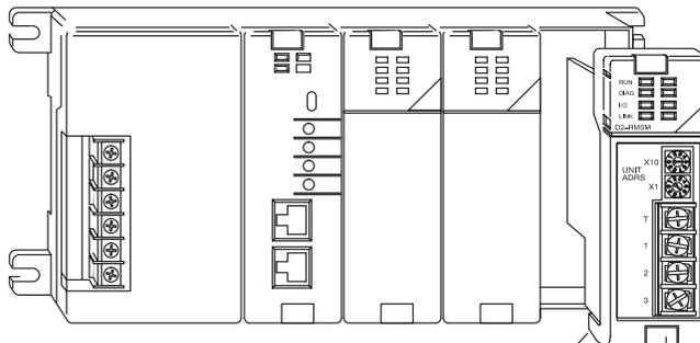
Align module to slots in base and slide inward
