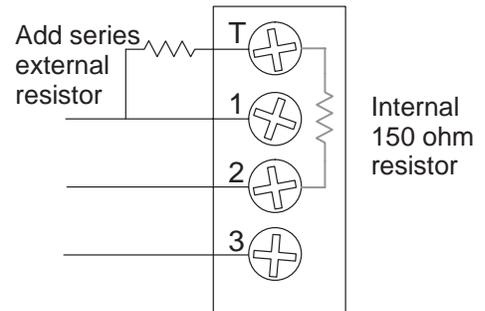
**Cabling Between the D3-350 CPU bottom port and Slaves**
