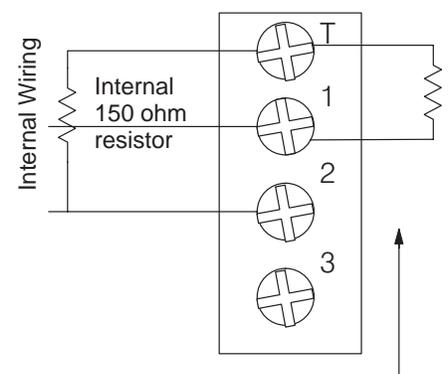
You use an external resistor in series with the internal resistor.
