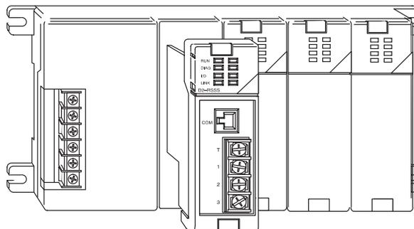
D2-RSSS must be in the CPU slot of the remote base.
