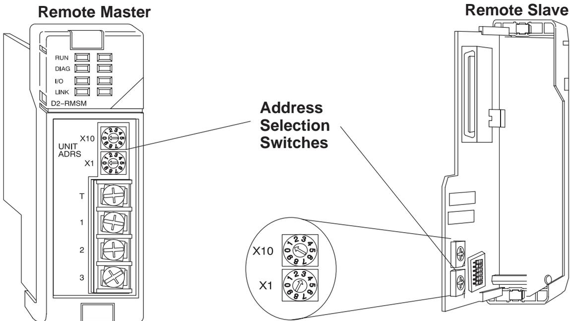
One switch is marked X1 and the other X10. Don't confuse these with the conventional data type labeling – *these do not refer to inputs X1 and X10*. Instead, these set the address in decimal for each unit. X1 is the “one's” position and X10 is the “ten's” position. For example, set address 13 by turning the X10 switch to 1 and the X1 switch to 3 (10+3=13).
