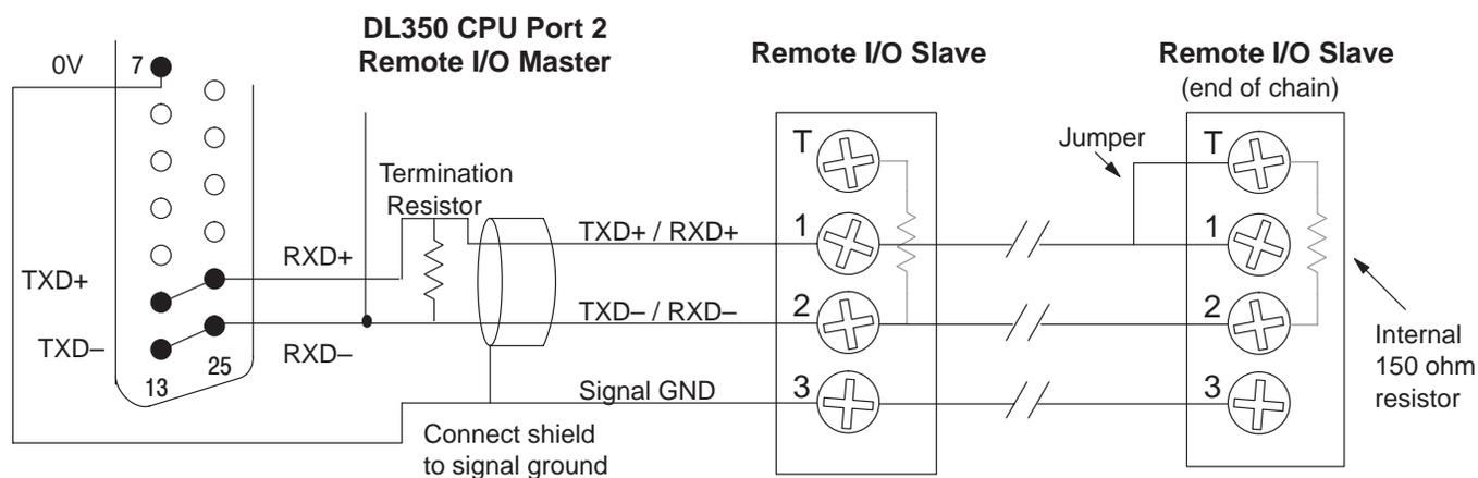
The twisted/shielded pair connects to the DL350's Port 2 as shown. Be sure to connect the cable shield wire to the signal ground connection. A termination resistor must be added externally to the CPU, as close as possible to the connector pins. Its purpose is to minimize electrical reflections that occur over long cables. Be sure to add the jumper at the last slave to connect the required internal termination resistor.
