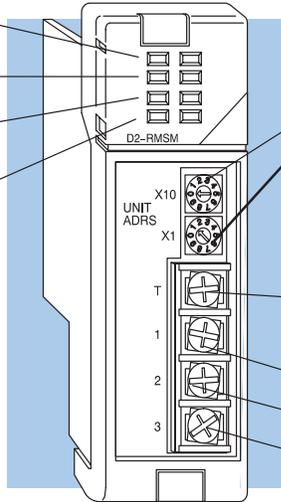
**UNIT ADDR**--Rotary switches for setting the module to be the master – always set to 0
