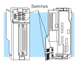
**STEP 4.** Install the D2–DCM in any slot except for Slot 0, which is next to the CPU.
