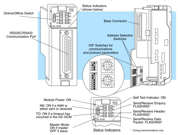
The DL205 Data Communications Module (D2–DCM) is a general purpose communications interface that can be used in a DL205 system that has a D2–240/250–1/260 Central Processing Unit (CPU). **The D2–DCM cannot be used with a DL230 CPU.** The module can go in any base slot, except for Slot 0, which is next to the CPU. This module is primarily used for three reasons.
