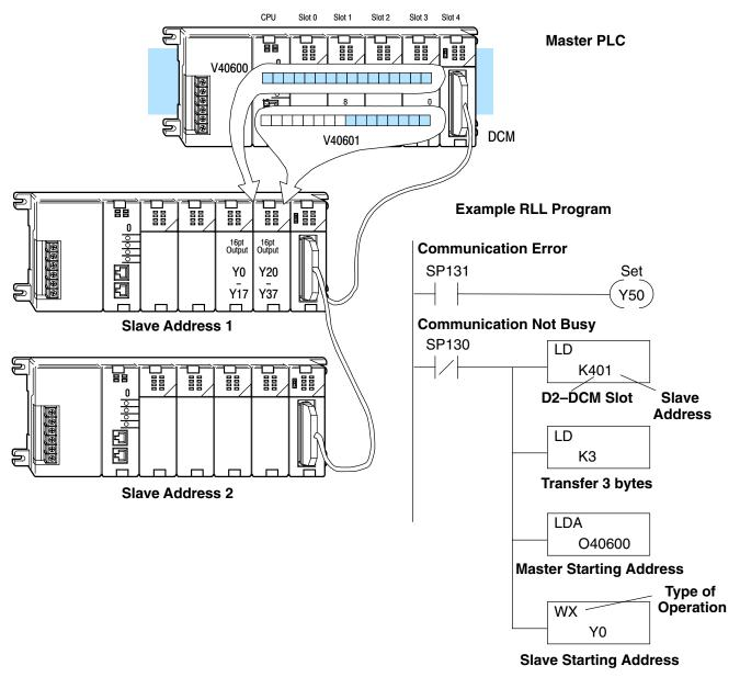
This example writes 3 bytes of data from the Master Station (starting at V40600) to Y0 - Y27 in Slave Station #1.
