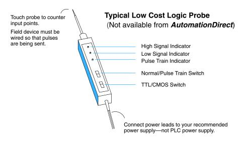
Check the specifications for the field device. Make certain that the output signal matches the specifications of the D2–CTRINT module.
