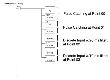
The hex number 5 stored in points 00 and 01 is the value for the Pulse Catching feature. Notice that the upper two digits of each hex value stored in V-memory for points 02 and 03 are the timing constants for filtering. The last two digits, 06, is the value for Discrete Filtered Inputs.
