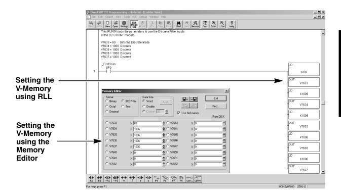
Editing the D2–CTRINT setup at the beginning of the user program is the most efficient method for setting up the counter mode. Should there be a need to change any of the counter setup values after the PLC has been put in the RUN Mode, use the Memory Editor to change the values. These values will only be temporary. They should be put into the program if they are to be used permanently.
