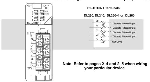
Shown in the above diagram and illustration are points 00 through 03 which default to discrete filtered inputs when the module is set for Mode 60.
