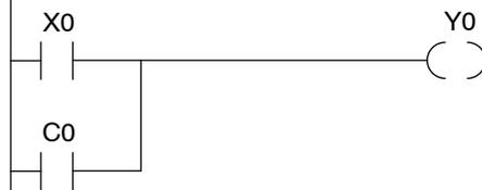
Y0 is normally controlled by X0 in the application. It is also controlled by C0 which is requested on during Bit Control, when the Change Preset Key is pressed.
