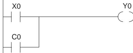
Y0 is normally controlled by X0 in the application. It is also controlled by C0 which is requested on during Bit Control, when the Change Preset Key is pressed.
