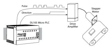
In the figure above, the DL105 generates pulse and direction signals. Each pulse represents the smallest increment of motion to the positioning system (such as one step or micro-step to a stepper system). Alternatively, the HSIO Pulse Output Mode may be configured to deliver counter clockwise (CCW) and clock-wise (CW) pulse signals as shown to the right.
