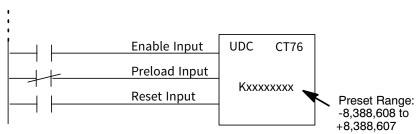
When the enable input is energized, the counter will respond to quadrature pulses on X0 and X1, incrementing or decrementing the counter at CT76 - CT77. The reset input contact behaves in a logical OR fashion with the physical reset input X2. This means the quadrature counter can receive a reset from either the contact(s) on the reset rung in the ladder, OR the external reset X2.
