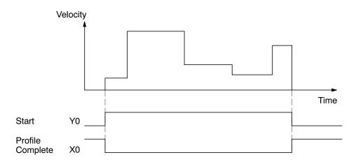
the velocity is set greater than zero, motion begins when the Start input (Y0) energizes. Since there is no end position target, the profile is considered in progress as long as the Start input remains active. The profile complete logical input to ladder logic (X0) correlates directly to the Start input status when velocity profiles are in use.
