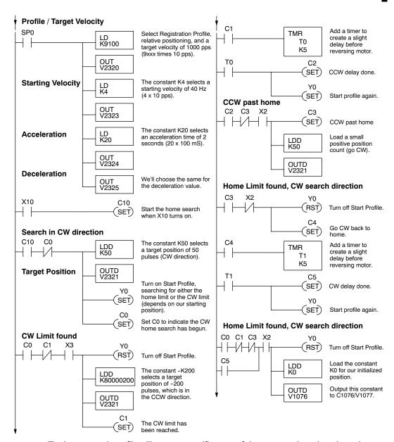
The home search profile will execute specific parts of the program, based on the order of detection of the limit switches. Ladder logic sets C0 to initiate a home search in the CW direction. If the CW limit is encountered, the program searches for home in the CCW direction, passes it slightly, and does the final CW search for home. After reaching home, the last ladder rung preloads the current position to "0".
