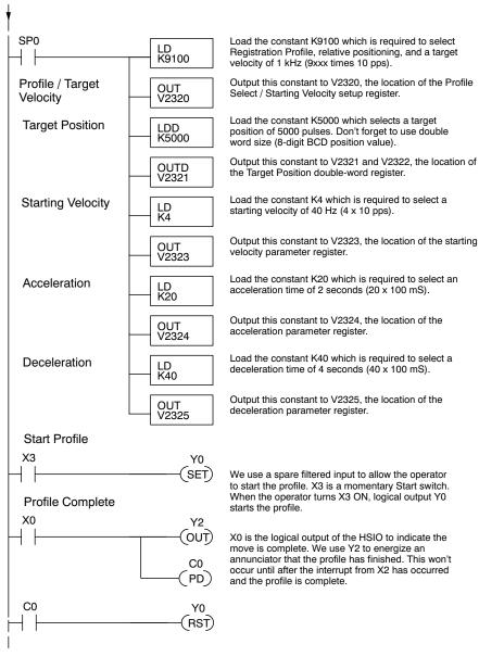
The profile will begin when the start input (X3) is given. Then the motion begins an indefinite move, which lasts until an external interrupt on X2 occurs. Then the motion continues on for 5000 more pulses before stopping.
