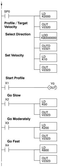
Load the constant K2000 which is required to select Velocity Profile. This data word contains no velocity information in the case of velocity mode.
