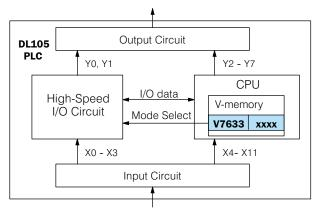
The contents of V7633 is a 16-bit word, to be entered in binary- coded decimal. The figure below defines what each 4-bit BCD digit of the word represents.
