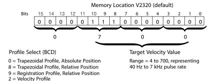
The ladder program must program this location before initiating any of the three profiles. The LD and OUT instruction will write all 16 bits, so be sure to fully specify the full four-digit BCD value for the Position / Velocity Select Register each time.
