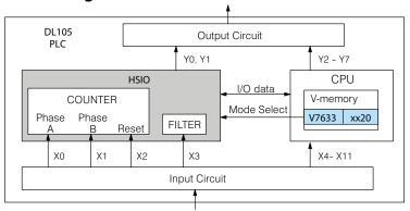
Quadrature encoder signals contain position and direction information, while their frequency represents speed of motion. Phase A and B signals shown below are phase-shifted 90 degrees, thus the quadrature name. When the rising edge of Phase A precedes Phase B's leading edge (indicates clockwise motion by convention), the HSIO counter counts UP. If Phase B's rising edge precedes Phase A's rising edge (indicates counter-clockwise motion), the counter counts DOWN.
