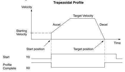
The HSIO uses logical output Y0 as the Start input to the HSIO, which starts the profile. Immediately the HSIO turns off the Profile Complete signal (logical X0), so the ladder program can monitor the progress of the move. Typically a ladder program will monitor this bit so it knows when to initiate the next profile move.
