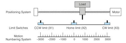
In the drawing above, the load moves left or right depending on the CCW/CW direction of motor rotation. The PLC ladder program senses the CCW and CW limit switches to stop the motor, before the load moves out-of-bounds and damages the machine. The home limit switch is used at powerup to establish the actual position. The numbering system is arbitrary, depending on a machine's engineering units.
