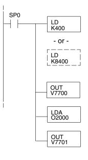
Loads a constant that specifies the number of channels to scan and the data format. The upper byte selects the data format (i.e. 0=BCD, 8=Binary) and the number of channels (set to 4 for the F0–04AD–2).
