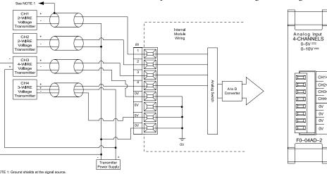
NOTE 1: Ground shields at the signal source. NOTE 2: Connect all external power supply commons.
