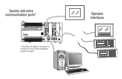
port to the master O/I(s) or PC(s). Port 1 and port 2 support slave mode operation.
