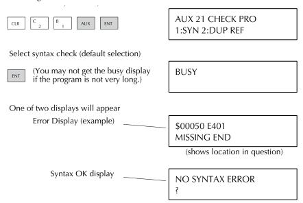
See the Error Codes Section for a complete listing of programming error codes. If you get an error, just press CLR and the Handheld will display the instruction where the error occurred. Correct the problem and continue running the Syntax check until the NO SYNTAX ERROR message appears.
