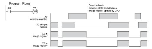
The following diagram shows how the bit override works for an output point. Notice the bit override maintains the output in the current state. If the output is on when the bit override is enabled, then the output stays on. If it is off, then the output stays off.
