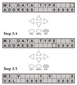
The data values on this screen will be four digits in length for BCD/HEX unless bit 8 of V7742 is set. Bit 8 of V7742 changes the data format to decimal (five digits).
