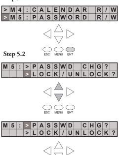
Use the up arrow or down arrow keys to scroll through number choices, and use the right arrow and left arrow keys to move from one digit position to another.
