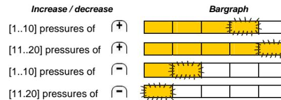
To save the new threshold value press white (SET) push-button or wait 30 sec. from last change (automatic save).
