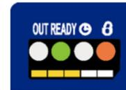
Increasing or decreasing the threshold, the right or left LEDs blink with a frequency proportional to the difference from the initial threshold value.
