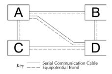
An equipotential bond wire must be provided alongside all serial communications cables, and to any separate items of the plant which contain I/O devices connected to the programmable controller. The diagram above shows an example of four physical locations connected by a communications cable.
