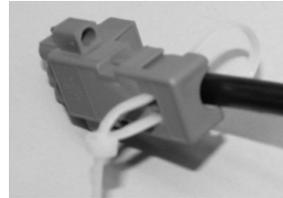
**Step 4:** Tighten the wire tie around the cable and the bottom shell.
