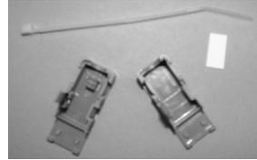
**Step 2:** Insert your pre-wired connector (with the screws facing up) into the bottom shell. (See manual for cable wiring instructions).
