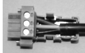
**Step 3:** Insert the wire tie from the bottom shell, loop around the cable and come back out of the opposite hole in the bottom shell.
