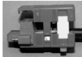
**Step 6:** Snap the top and bottom shells together.
